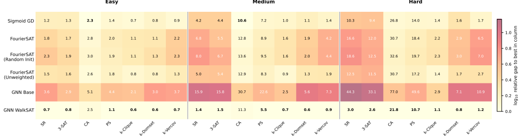
Figure 3: Direct GD and FourierSAT-style optimization on the mixed G4SATBench split. Cell annotations show mean final expected unsatisfied clauses and color shows the \log_{10} relative gap to the best method in each column. Lower values and lighter cells are better.
